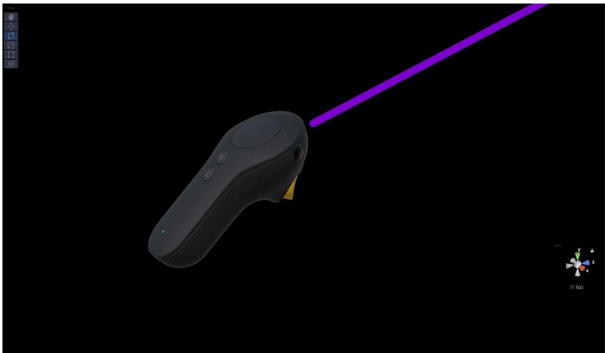
**Figure 53: 3D model of the controller with the ray for interacting with the UI and the available button highlighted in yellow color.**
